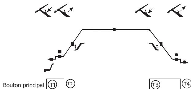
T1: The main button is pressed, the cycle starts at PreGas and stops in the I\_Start phase.
