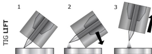
1. Position the torch nozzle and the electrode tip on the workpiece and press the torch button.
