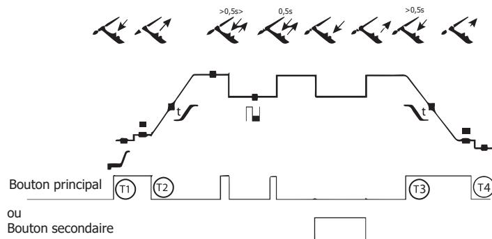
T1: The main button is pressed, the cycle starts at PreGas and stops in the I\_Start phase.
