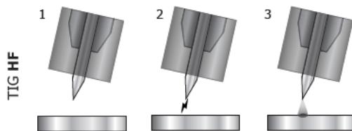
1. Place the torch in the welding position above the part (distance of about 2-3 mm between the electrode tip and the part).
