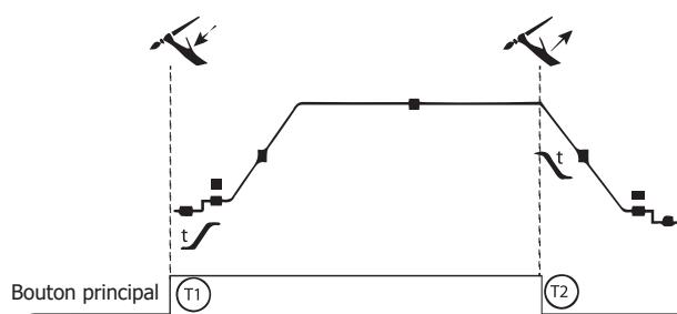
T1: The main button is pressed, the welding cycle starts (PreGas, I\_Start, UpSlope and welding).
