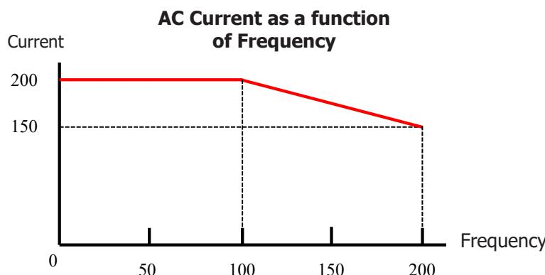
Up to 100 Hz it is possible to weld at a welding current of 200 A. Between 100 Hz and 200 Hz, the maximum value of the welding current decreases from 200 A to 150 A.
