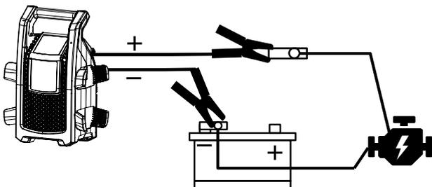
Disconnect the (+) terminal from your battery and connect the red (+) clamp of the GYSCAP 680E to it. Connect the black (-) clamp to the (-) terminal of your battery.
