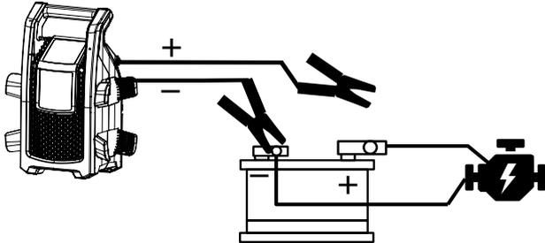
Remove the red clip (+) from the terminal attached to the battery.
