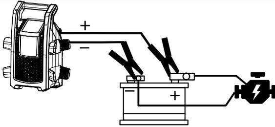
Replace the assembly: terminal and red (+) clip on the (+) terminal of the battery.
