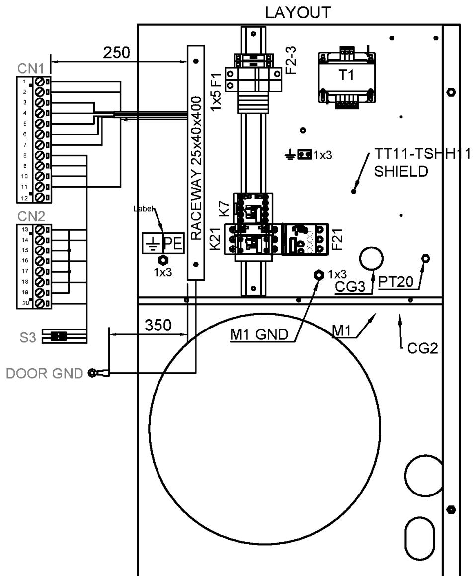
**28.5 - Cubicle components (NS 4, NS 5.5, NSD 4, NSD 5.5) - ASME - (380V, 460V) - DOL**
