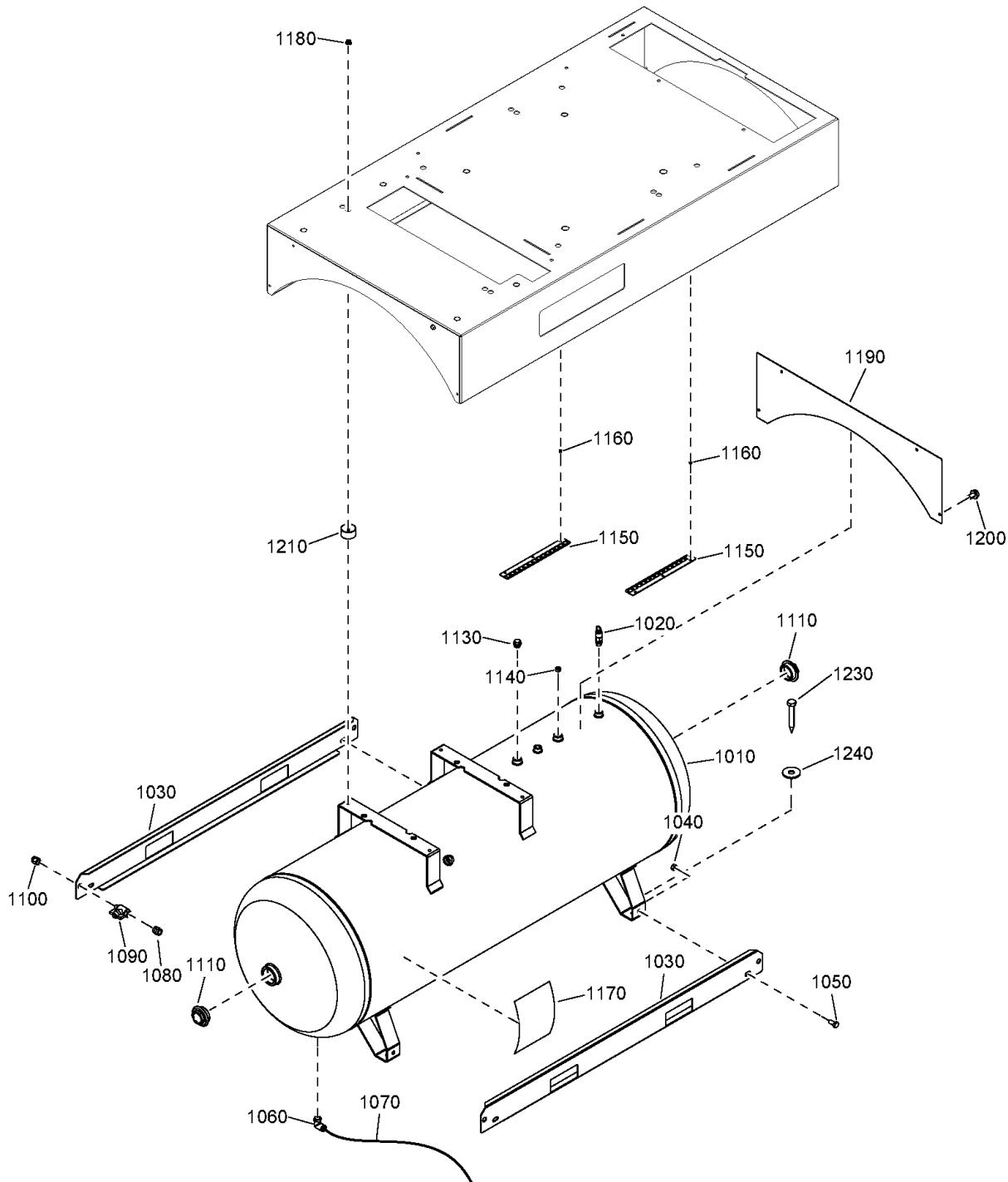
**24 - Air vessel (NSD 7.5, NSD 10) - (CE, CEAD2000) - Air receiver - 500L - With dryer**
