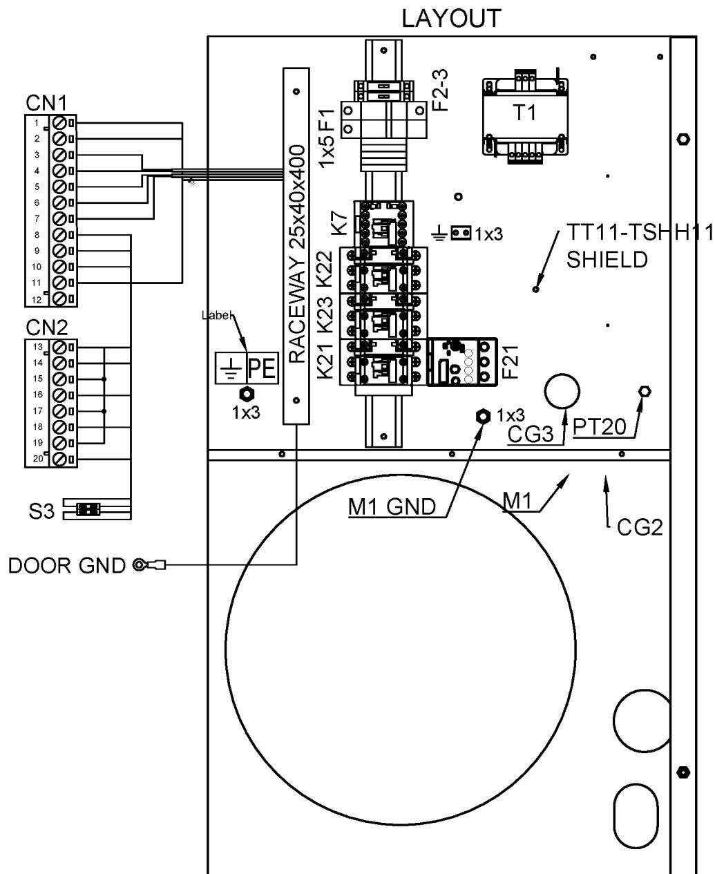
**28.6 - Cubicle components (NS 5.5, NS 7.5, NS 10, NSD 5.5, NSD 7.5, NSD 10) - (ASME, CE, CEAD2000) - 230V - YD**
