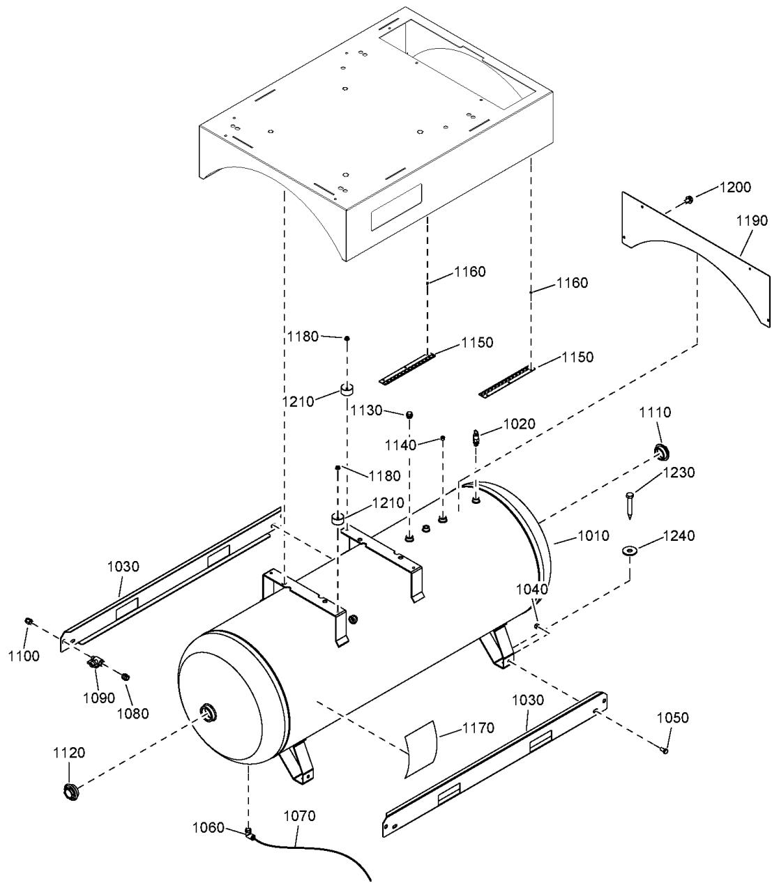
**20 - Air vessel (NSD 7.5, NSD 10) - (CE, CEAD2000) - Air receiver - 500L - Without dryer**
