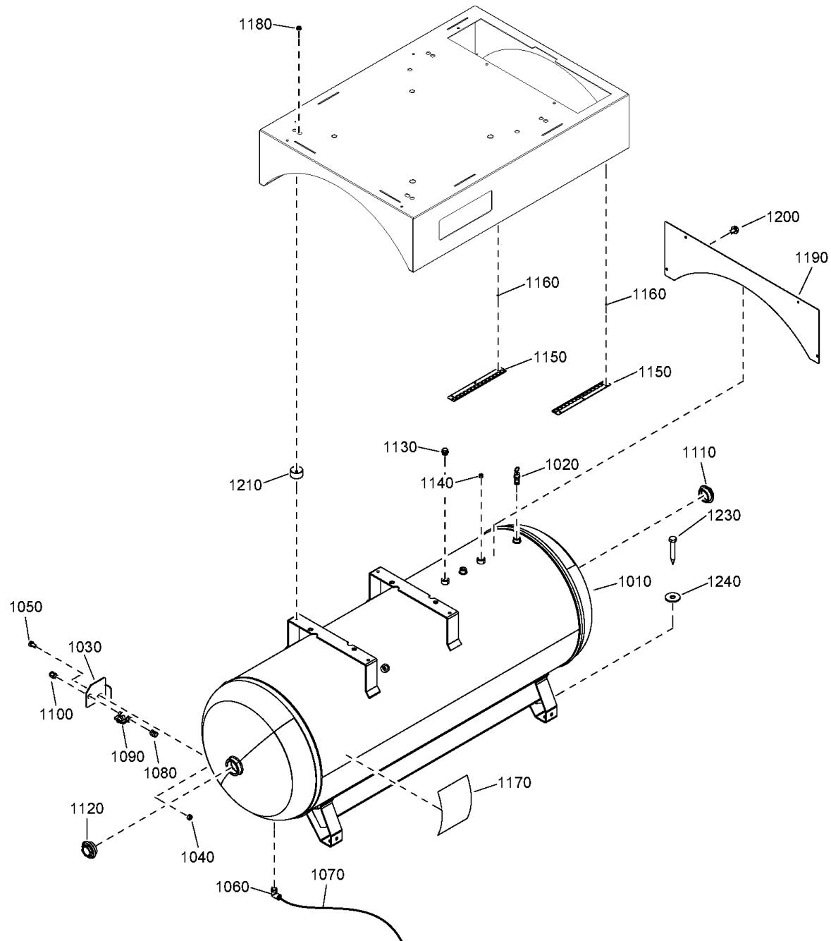
**22 - Air vessel (NSD 7.5, NSD 10) - ASME - Air receiver - 500L - Without dryer**
