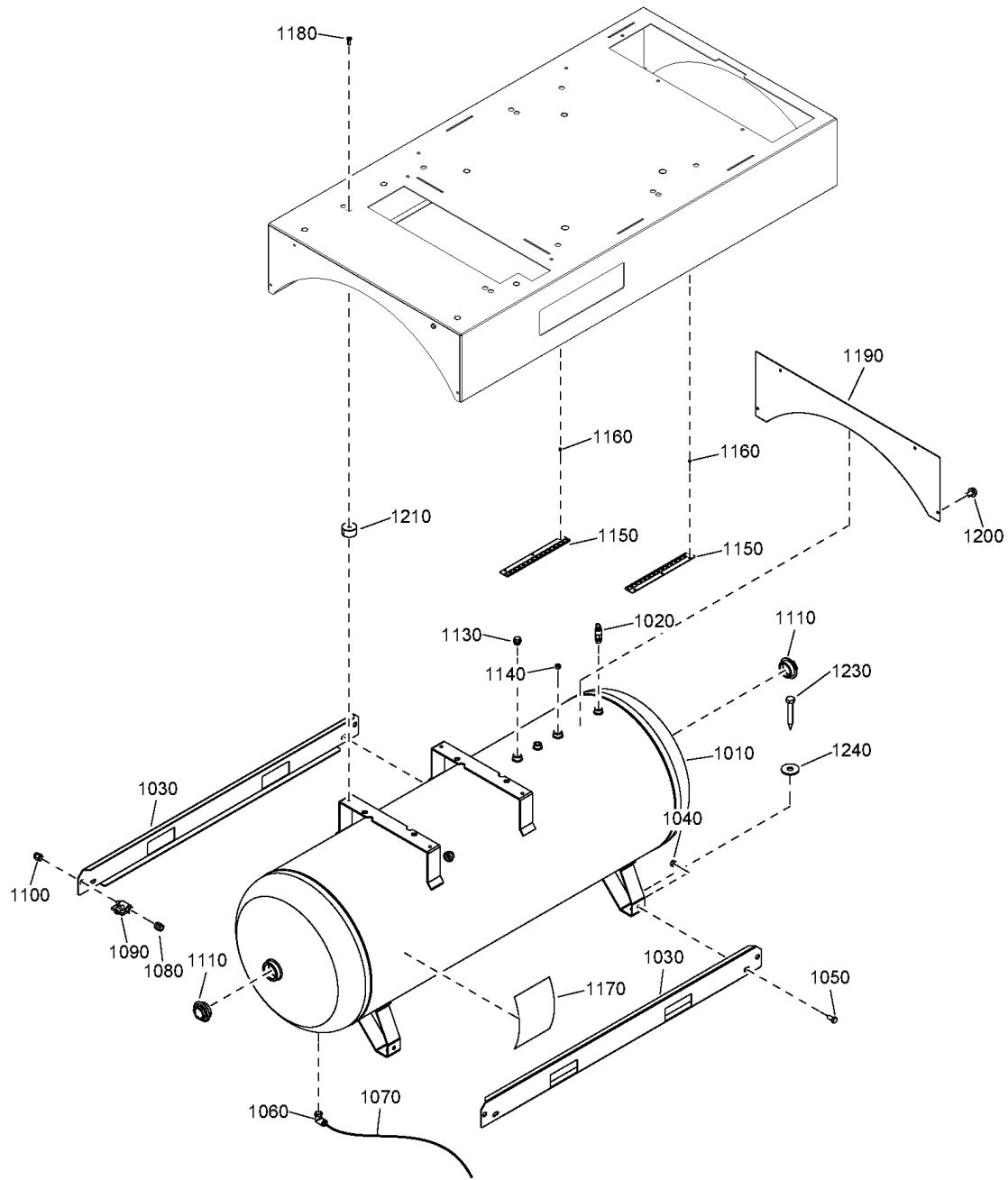
**23 - Air vessel (NS 7.5, NS 10) - (AS1210, CE, CEAD2000, MOM) - Air receiver - 500L - With dryer**
