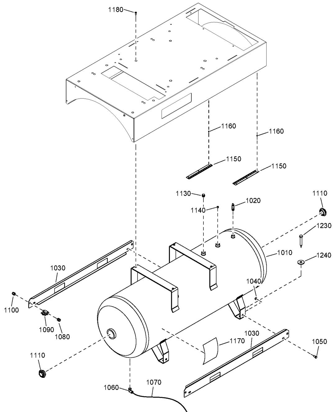
**18 - Air vessel CE, MOM, AS1210, CEAD2000 - Air receiver - 270L - With dryer**
