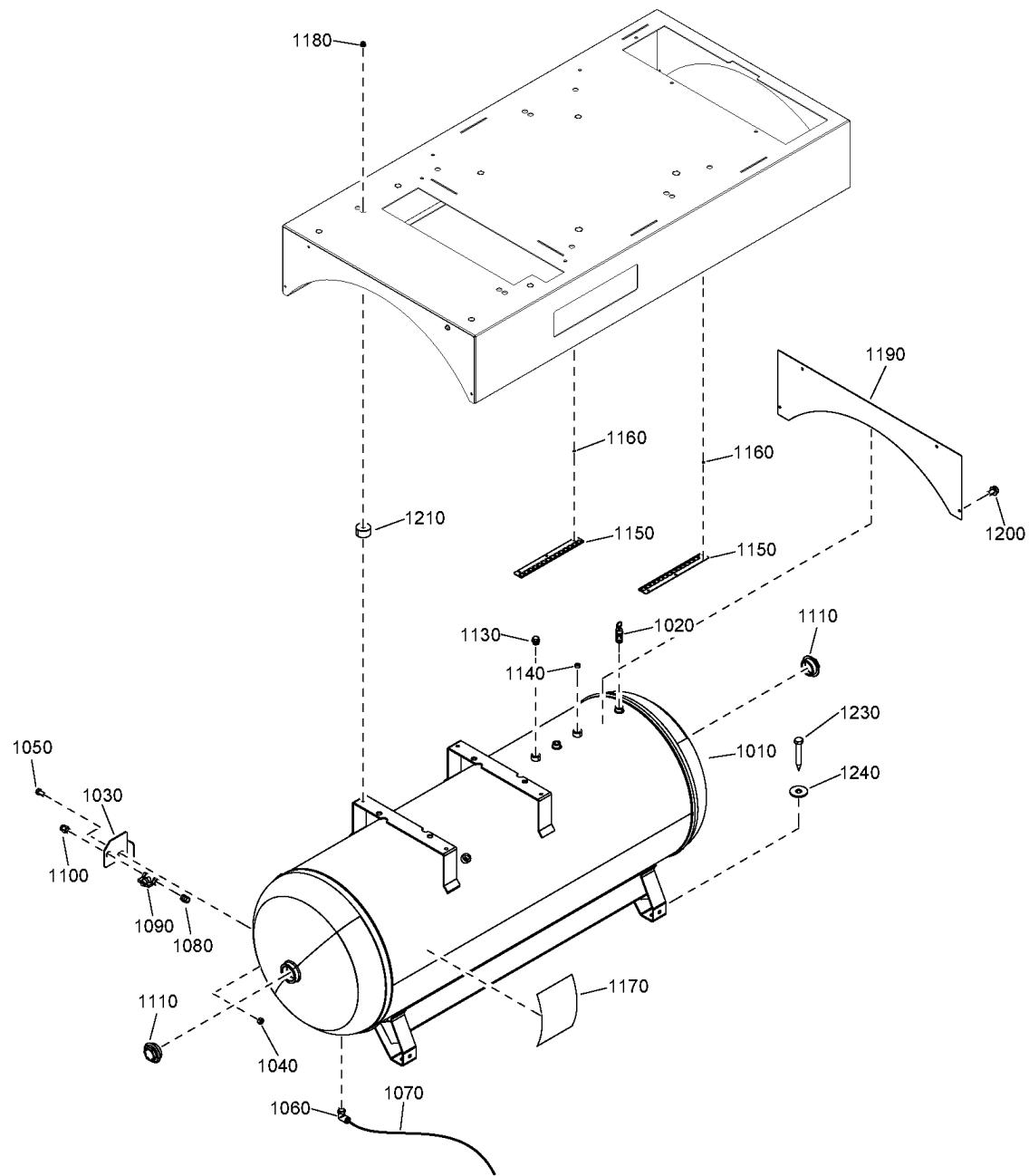
**26 - Air vessel (NSD 7.5, NSD10) - ASME - Air receiver - 500L - With dryer**
