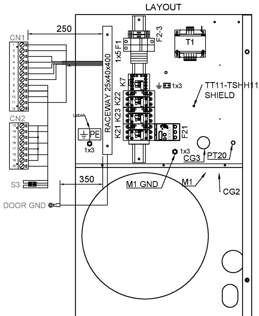
**28.8 - Cubicle components (NS 5.5, NS 7.5, NS 10, NSD 5.5, NSD 7.5, NSD 10) - ASME - (380V, 460V) - YD**
