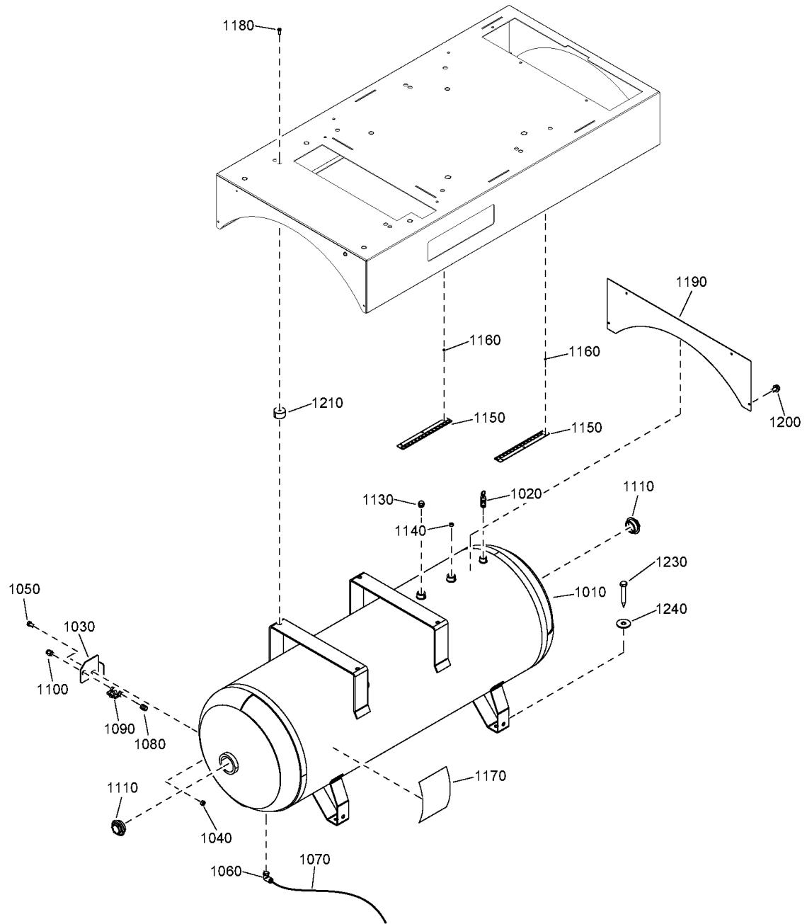
**25 - Air vessel (NS 7.5, NS 10) - (ASME, CRNASME) - Air receiver - 500L - With dryer**
