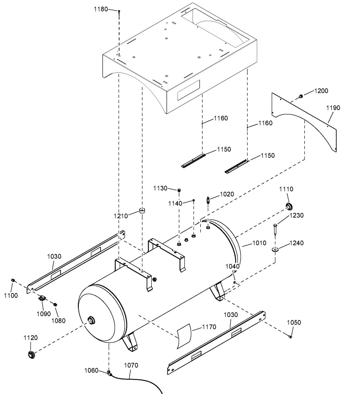
**19 - Air vessel (NS 7.5, NS 10) - (AS1210, CE, CEAD2000, MOM) - Air receiver - 500L - Without dryer**
