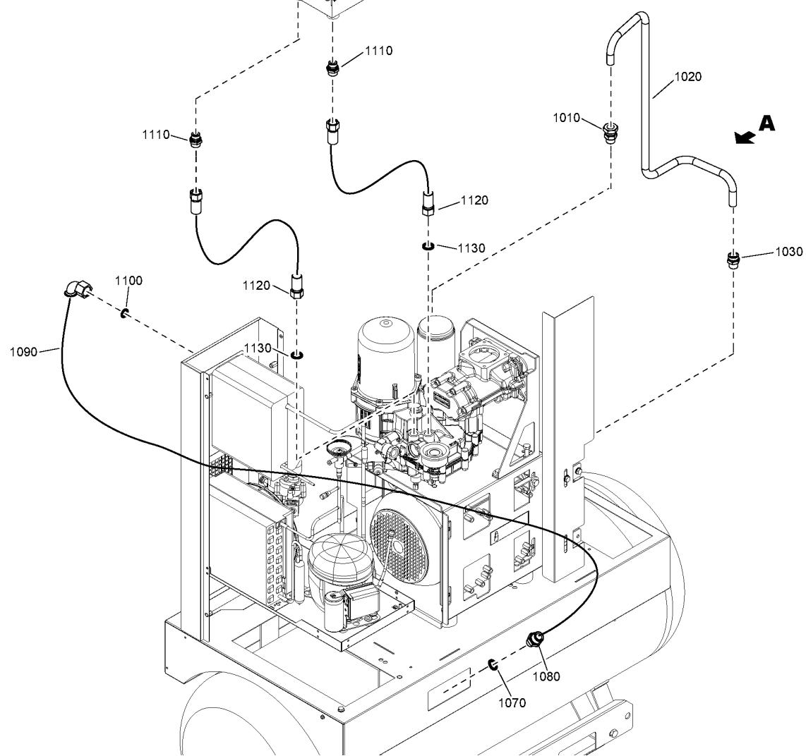
**10 - Fluid transportation Tank-mounted - With dryer**
